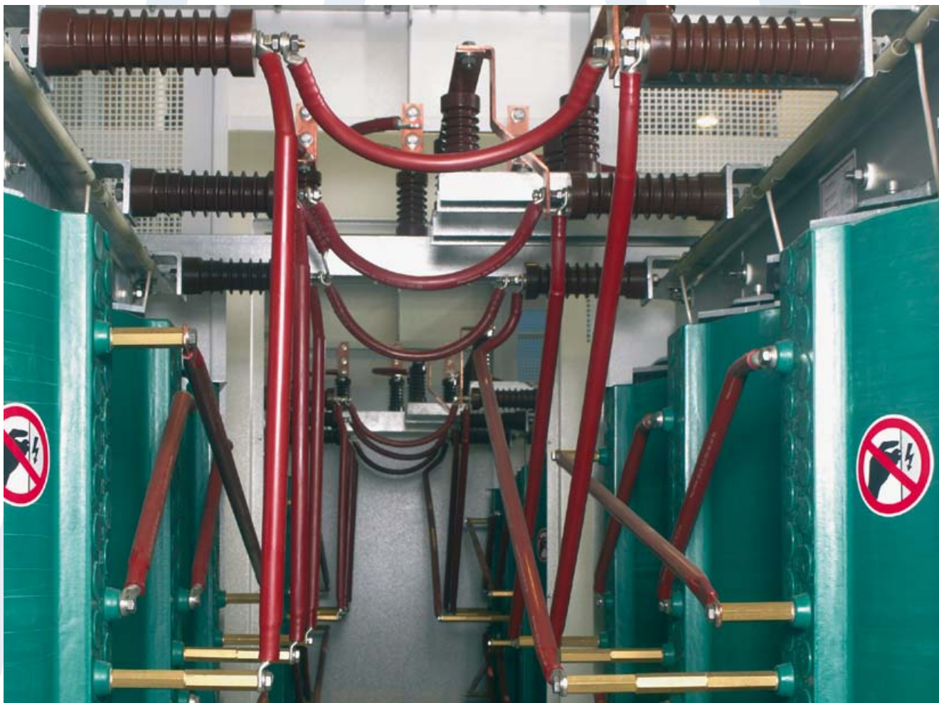
946 kVA 10kV / 2x700V DTR 101000 12 pulse rectifier transformer with phase shift \pm 7,5^\circ
